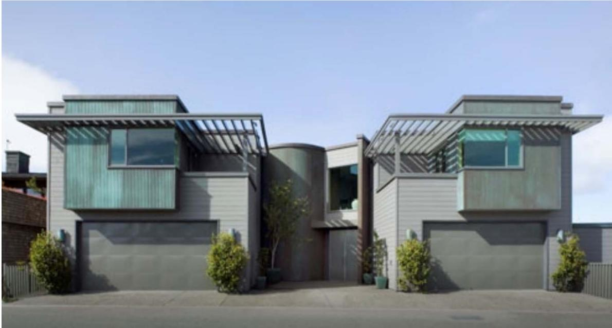
*The street elevation offers little about the views. The exterior materials are stained resawn red cedar and verdi-gris corrugated copper siding.*
