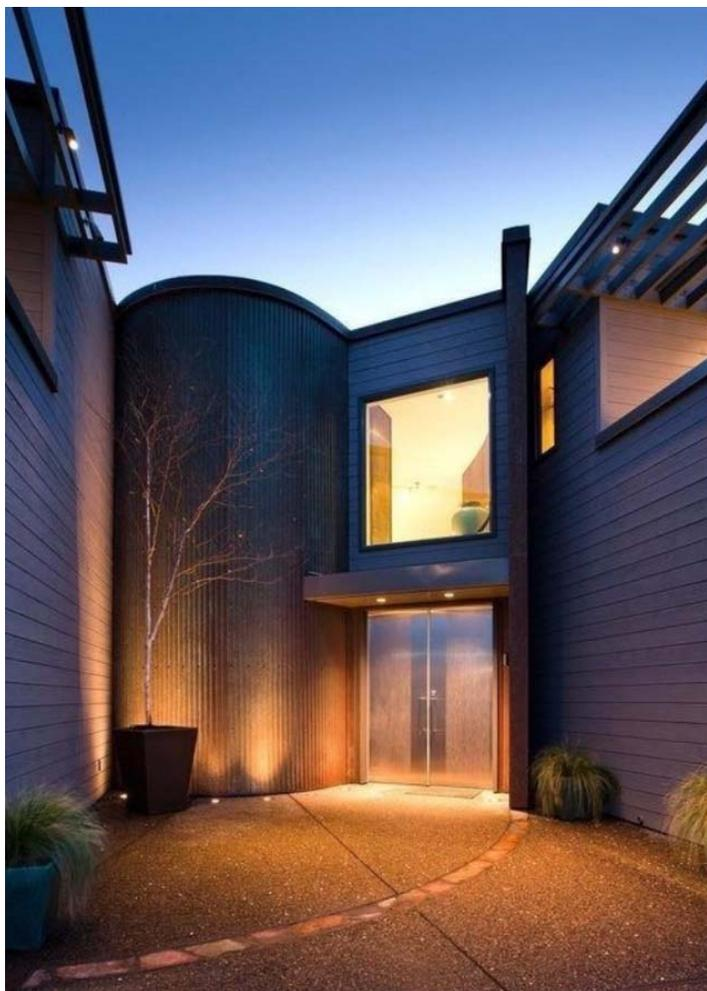
*The entry courtyard leads to stainless steel doors. The curved corrugated copper wall contains the shell-shaped stairs*
