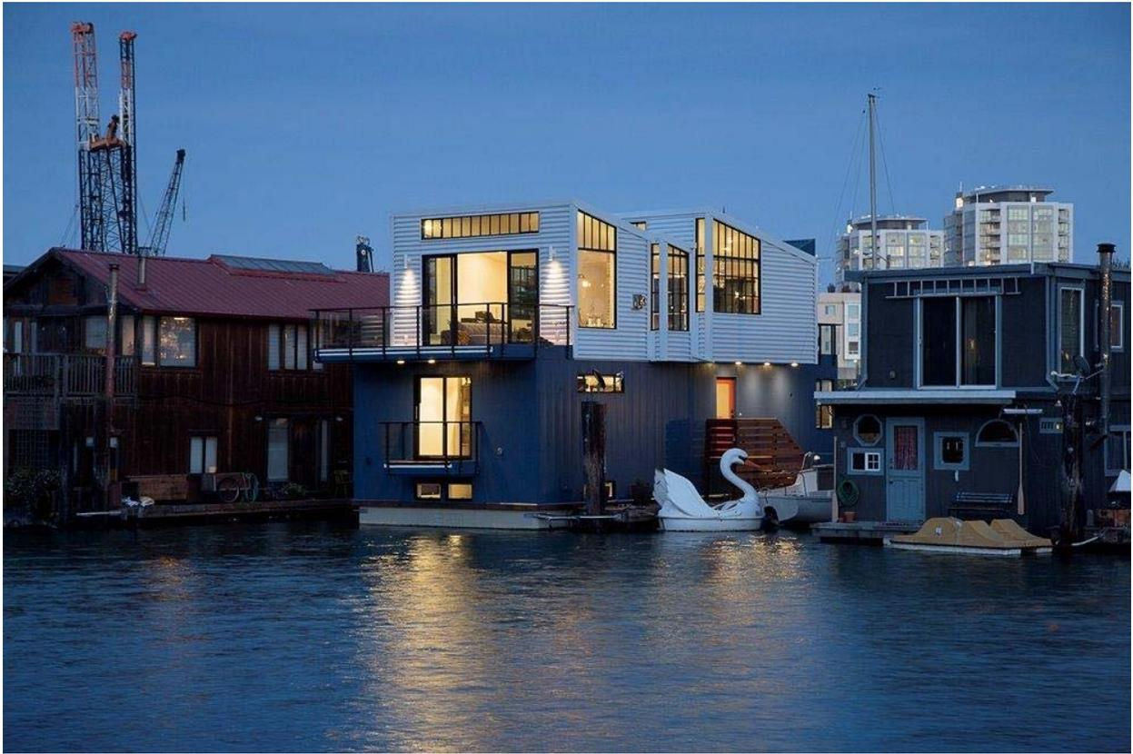
Made of black anodized aluminum with stainless steel hinges, the home's warehouse-style windows are designed to withstand corrosion. No wood was used on the exterior except for the dock, called a finger pier, which allows access to the front door and the couple's boat. The home looks out onto downtown San Francisco, with AT&T Park visible from the main deck. The Swan boat was once of many a ride at a nearby water park many years ago.
